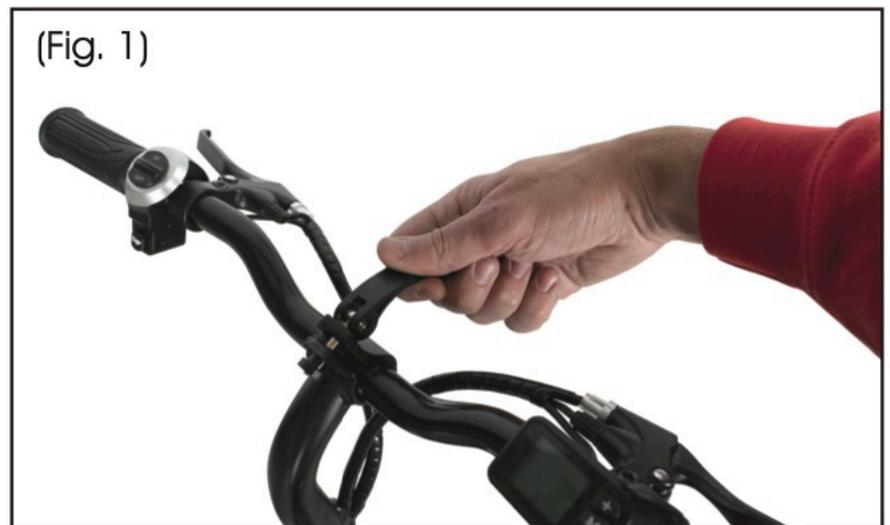
Once the handlebar is attached, unlock the stem assembly and fold it down again to expose the interior bolt.
