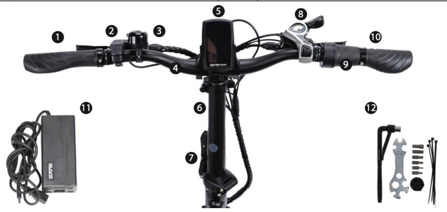
The LED display is Waterproof IPX6-rated, whichmeans that it will repel a significant, sustained rainstorm without any issues.
