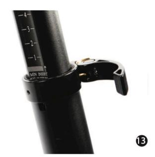
**NOTE:** The seat post has a "Minimum Insertion Mark" stamped onto it, which is shown by the knurling on the tube (13). These marks must always be BELOW the top of the seat tube of the bicycle frame. If the bicycle is ridden with these marks above the seat tube, the seat post can unexpectedly bend or break due to the leverage being placed on it by the weight of the rider. Failure to insert the seat tube properly into the frame can cause injury and/or damage to the bicycle frame and components.
