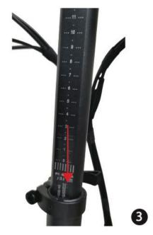
**WARNING:** The upper handlebar assembly has a "Minimum Insertion Mark" printed onto it (3). This mark must always be BELOW the lower handlebar assembly clamp. If the bicycle is ridden with these marks above the clamp, the upper handlebar assembly can unexpectedly bend or break due to the leverage being placed on it by the rider. Failure to insert the upper handlebar assembly properly into the lower handlebar assembly can cause injury and/or damage to the bicycle frame and components.
